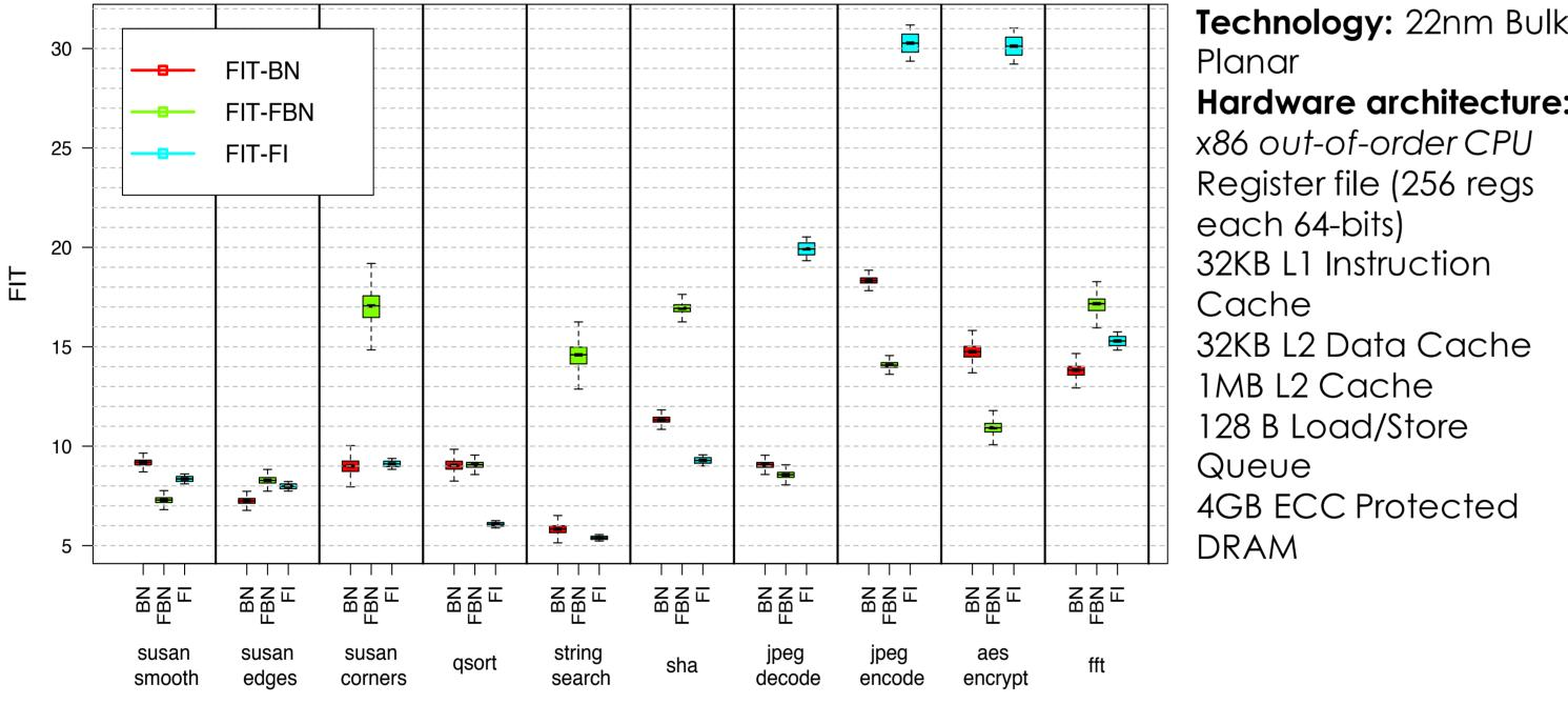
FIT estimation for a x86 based system running 10 software benchmarks: (1)  $FIT_{BN}$ computed with the CLERECO model, (2) FIT<sub>FBN</sub> computed with the CLERECO model using average masking probabilities, (3) FIT<sub>FI</sub> computed using full fault injection campaigns
