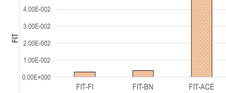
through ACE analysis for the string search benchmark computed with technology: FIT<sub>BN</sub> computed with the CLERECO model, FIT<sub>FI</sub> computed using full fault injection campaigns, FIT<sub>ACE</sub> computed using ACE analysis with literature data
