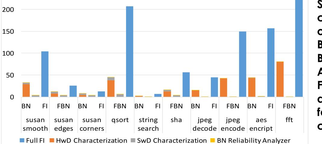
Simulation time comparison in hours of simulation: **BN: CLERECO Bayesian Reliability** Analyzer FI: full micro architectural level fault injection campaign.
