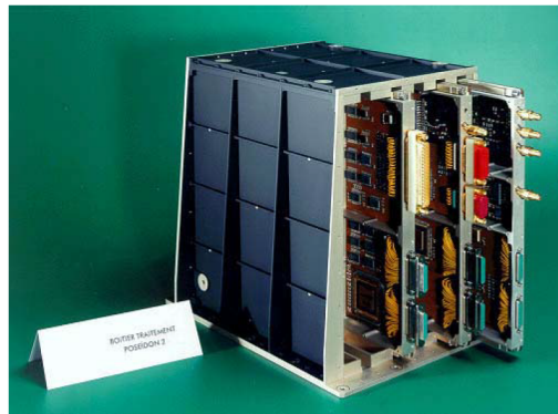
Figure 7: Example of processing unit (on-board the Poseidon-2 satellite).
