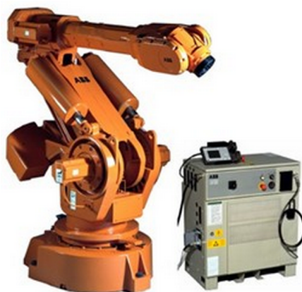
Figure 7 - Robot with control system
